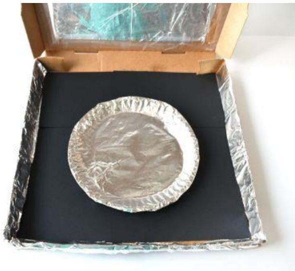
8. Place an aluminum pie pan or a plate covered with aluminum foil inside your new solar oven.
