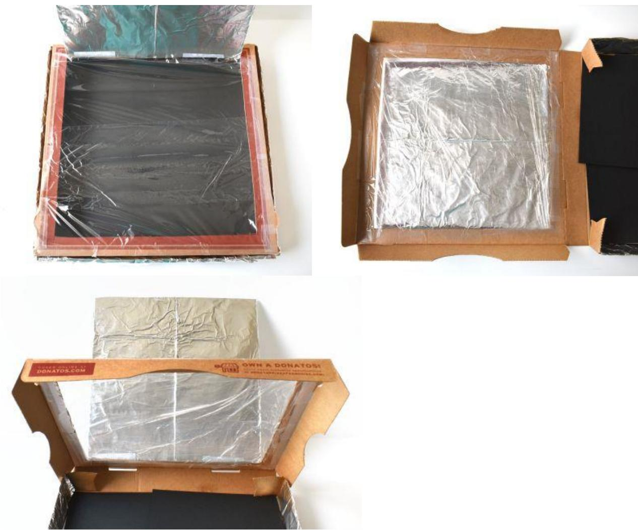
7. Now you'll need to cover the opening with plastic wrap. Securely tape one piece of plastic wrap to the top of the hole and one piece underneath the hole. You want to create an airtight window.
