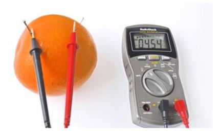
Turn on the voltmeter. If you are using a multimeter, make sure it is set to measure volts.
