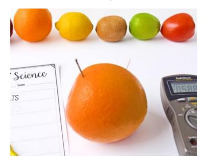
Insert the piece of copper into the fruit. Then, insert the nail into the fruit at least an inch away from the piece of copper. If you insert them at an angle, make sure that the pieces do not touch each other inside the fruit.
